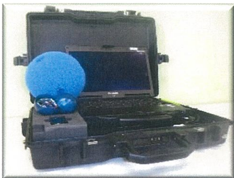
Figure 2: SmartBall Core, Foam Outer Shell & SBRs
