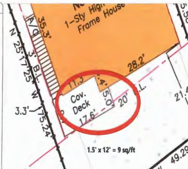
Blow up of encroachment
